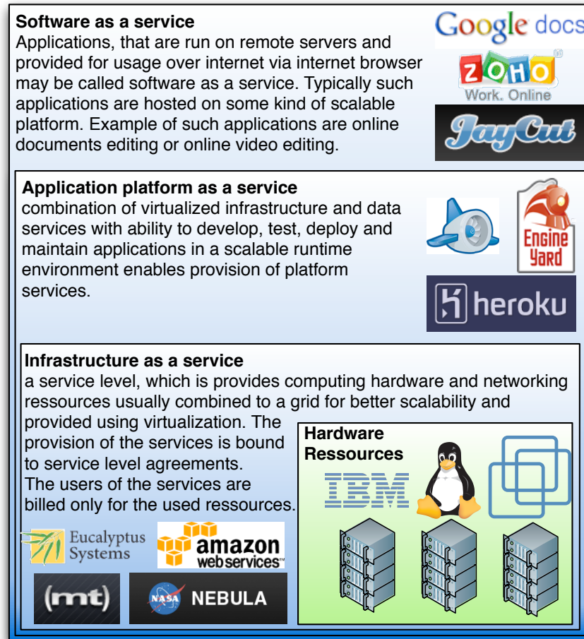
Figure 1.1.: This image shows the hierarchy of three levels of cloud computing services - software as a service, platform as a service and infrastructure as a service.
