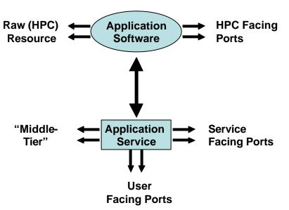
Figure 2. A Proxy Service Programming Model showing 4 types of Interactions :to and from users (portal interface), between proxy and raw resource, other middle-tier components and between other raw (hpc) resources
